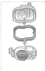
Steam cap exploded view
