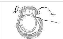
③ Disassemble the rubber packing in the direction of the arrow.
