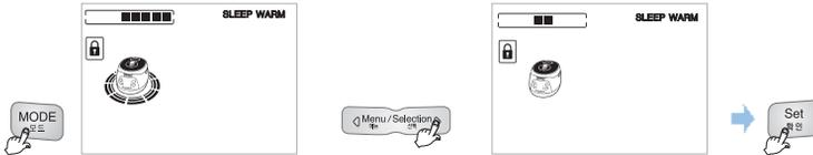
1. Hold “the mode” button for one second, then press the “mode” button 6times to set up sleeping mode. If sleeping mode is not shown, keep on pressing the “mode”button until it is heard or displayed.
