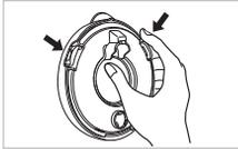
❷ Disassemble soft steam cap in the rear by pressing the hook in direction, at the arrow and wash it frequently with an neutral detergent and sponge.
