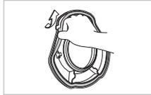
❸ Disassemble the rubber packing in the direction of the arrow.
