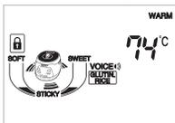
If you push the “set” button present warming temperature is displayed and push “set” button again. The current time is displayed during warming. Moreover, when you push the button once more, the time elapsed of warming is displayed
