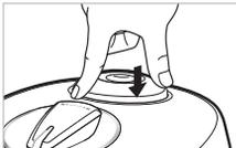
❻ When installing the soft steam cap, insert the cap firmly by pressing in the direction of the arrow indicated in the figure.
