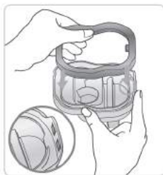
1. As shown in the picture, fit the rubber gasket into the groove and insert it.
